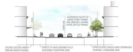
Figure 13 Cross section depicting general street network and design guidelines.
